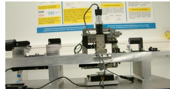
Test setup for the CCD Microscope
