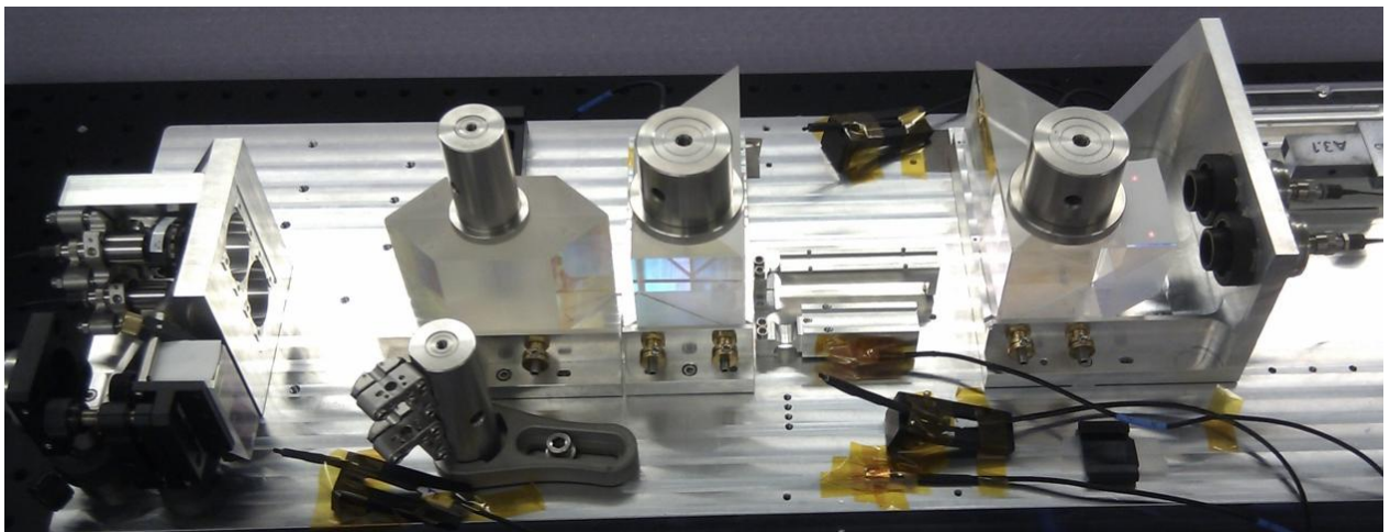
Figure 1. Picodrift interferometer with, in the center between the two main polarising beam-splitters, the sample and refractometer cell holder.
