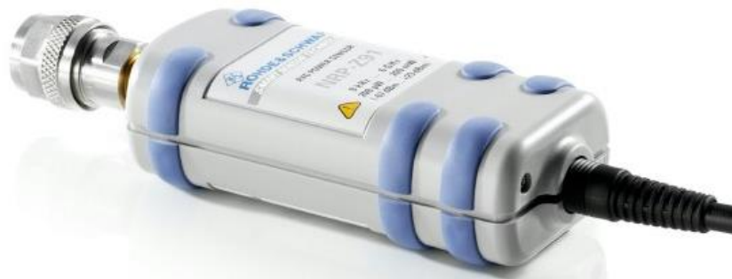
Figure 4: R&S NRP-Z91 Average Power Sensor. It has a multi-diode technology which gives it a very large dynamic range. This is achieved by splitting the measurement voltage among several diodes. So that each diode is driven exclusively in the square law region and each diode is driven less 3 .
