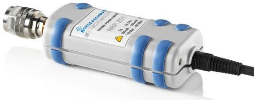
Figure 2: R&S NRP Z51 Thermal power sensor. It has a frequency range from DC – 18GHz and dynamic range from -35dBm to 20dBm 2
