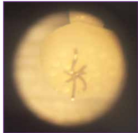
Fig 1. A wad shaped (b) differential thermo-couple (DTC) [as intermediate state in the development], one of several used within the SR5 – System developed by Dr. Ernst Lenz and his colleagues at PTB that include planar shaped (a) and in the final stage point shaped (c) examples. All stages [b), c)] are accompanied by a reduction of the electrical uncertainty by simultaneously preserving good thermal contact.
