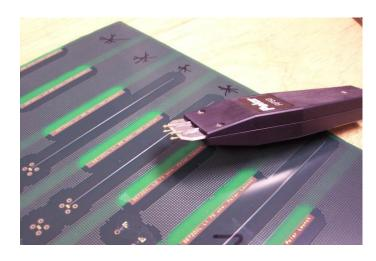
Traceable Differential S-parameter Measurements on Planar Circuits to Test Signal Integrity
