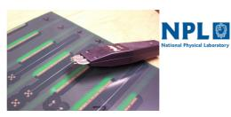
Traceable Differential S-parameter Measurements on Planar Circuits to Test Signal Integrity
