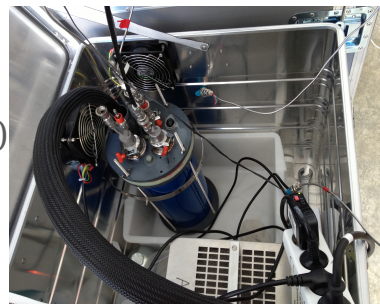
-60°C drying system, with Mg(ClO 4 ) 2 trap follow-up
