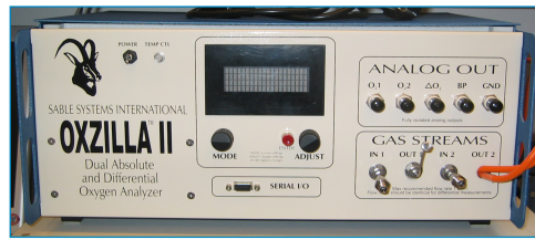
the heart of the system: "differential" fuel cell oxygen measurement system
