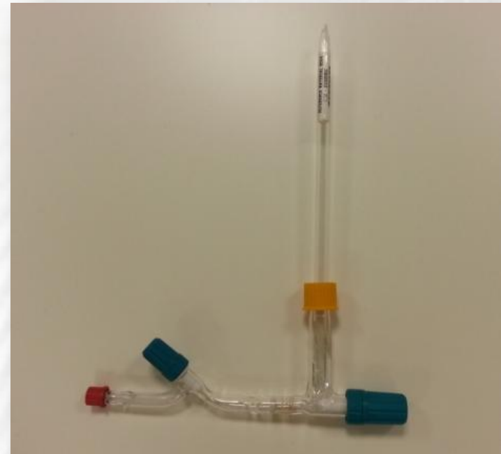
Tube cracker at TÜBİTAK UME
