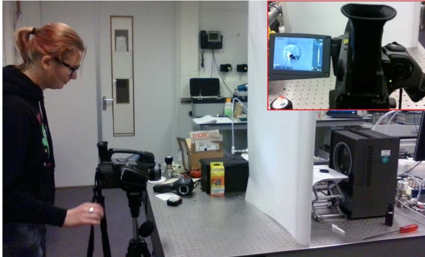
Test of the infrared camera in the laboratory. In front of a blackbody radiator a small cup containing liquid methanol is shown. The white plastic is transparent for infrared radiation. The inset shows the picture taken by the camera.
