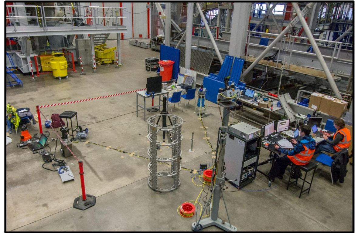
Test setup at Airbus with 4 sensor heads and 12 targets
