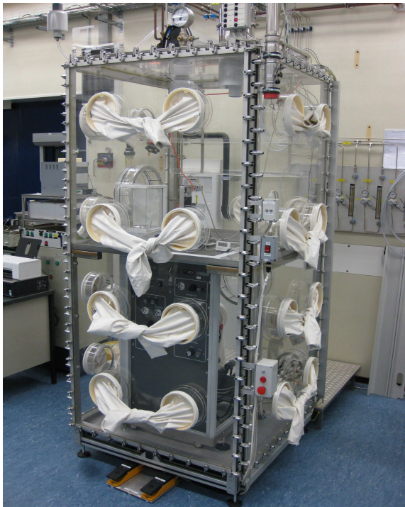
Fig. 4. The drop calorimeter installed inside a glove box
