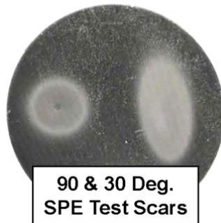
Figure 7 Example of the effect of different angles of incidence in erosion testing.
