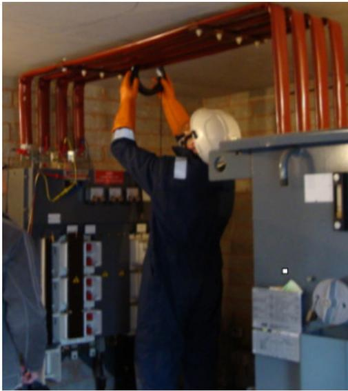
Site Measurement in substation: Fitting Rogowski coil to a live bus bar
