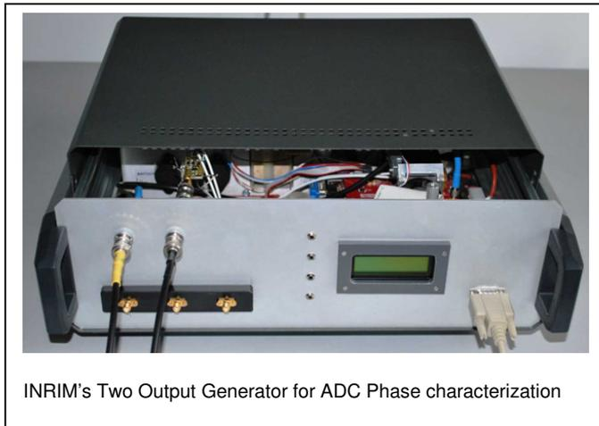
INRIM's Two Output Generator for ADC Phase characterization
