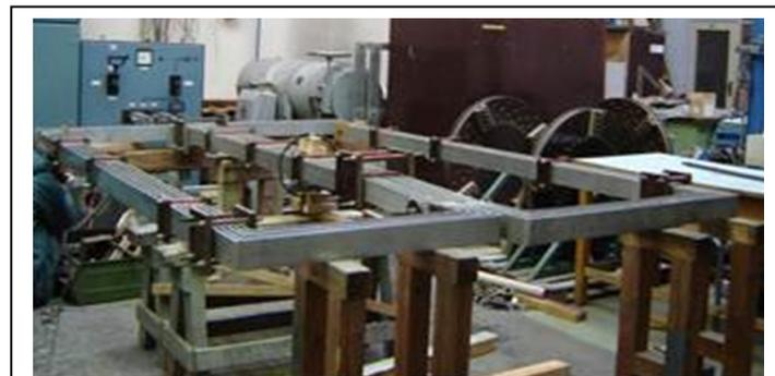
Current loop for the calibration of Rogowski coil up to 30 kA
