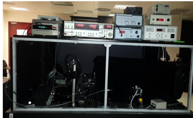
Fig. 14 DSR System established at TUBITAK for calibrating solar cells.
