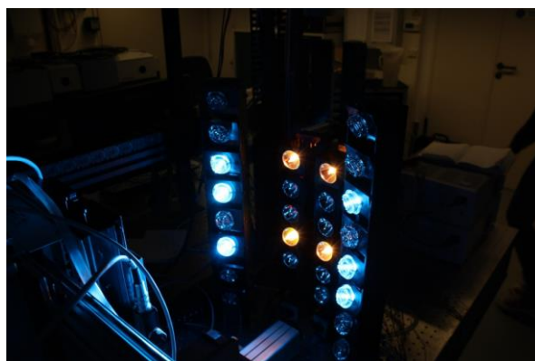
Fig. 13 Bias lights working at AM0 like conditions.
